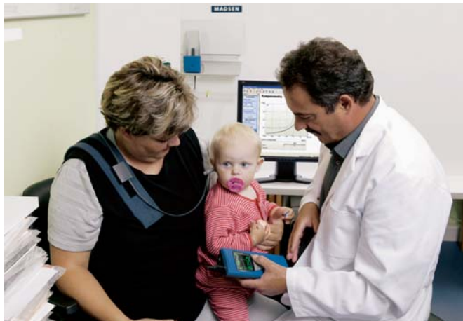
Figure 4. A infant referred from a neonatal screening program is measured with a 1000-Hz probe tone using the MADSEN OTOflex 100 from GN Otometrics.
